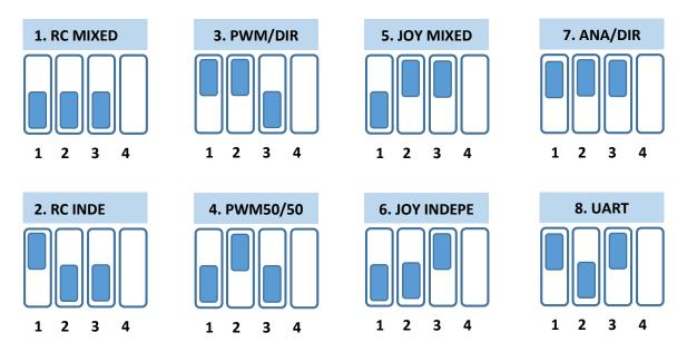
When power on **or** changing mode. The Run LED in the PCB will blinking a X sequence number to confirm witch mode are configured. X = 1 (PWM 50/50), X=2 (PWM/DIR),..., X=6 (ANA/JOY)
