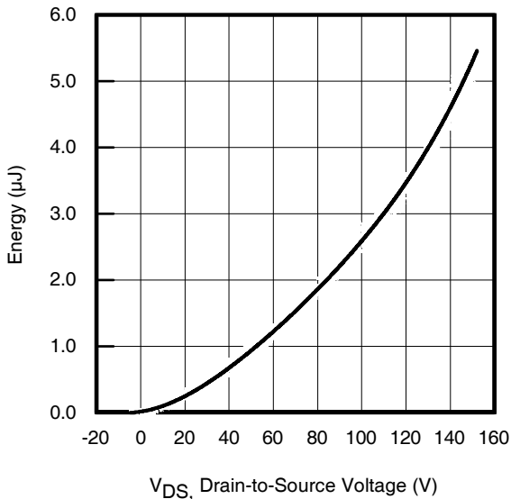
Fig 11. Typical C_{OSS} Stored Energy
